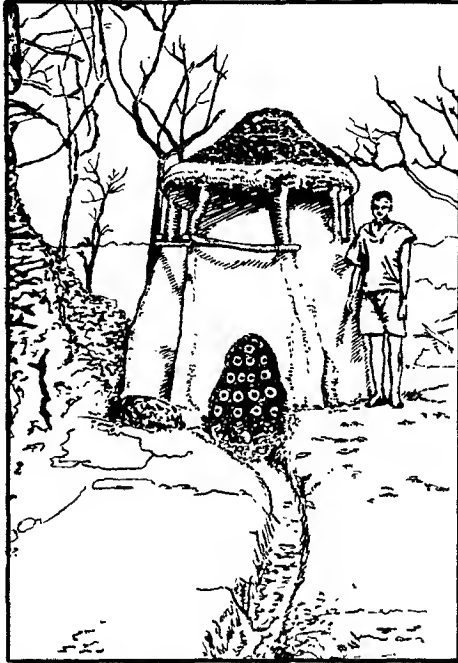
Fig. 7. Furnace: BaUshi. The furnace charged with ventilating tubes in place (redrawn from 13).
